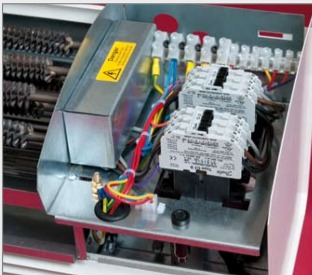
Electrical connections box
